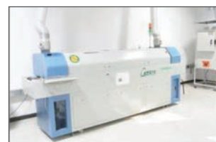
For SMD type products, simulating IR RELOW testing / 高溫無鉛回流焊機 (晉力達)
